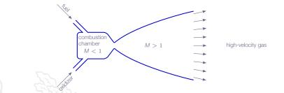
High-temperature, high-pressure gas in combustion chamber expand through the nozzle to very high velocities. Typical figures for a LH<sup>2</sup>/LOx rocket engine:  $p_o \sim 120$  [bar],  $T_o \sim 3600$  [K], exit velocity  $\sim 4000$  [m/s]
