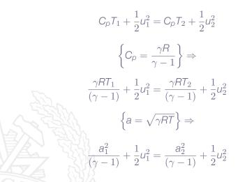
In any position in the flow we can get a relation between the local speed of sound *a*, the local velocity *u*, and the speed of sound at sonic conditions  $a^*$  by inserting in the equation on the previous slide.  $u_1 = u$ ,  $a_1 = a$ ,  $u_2 = a_2 = a^* \Rightarrow$
