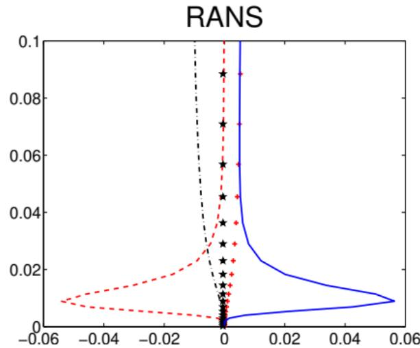
$\text{---} : \frac{\partial}{\partial y} (2\langle \nu_t \bar{s}_{12} \rangle)$ ;  $\text{---} : \nu \frac{\partial^2 \langle \bar{u} \rangle}{\partial y^2}$ ;  $\text{---} : -\frac{\partial \langle \bar{u} \rangle \langle \bar{u} \rangle}{\partial x}$ ;  $+ : -\frac{\partial \langle \bar{u} \rangle \langle \bar{v} \rangle}{\partial y}$ ;  $* : -\frac{\partial \langle \bar{p} \rangle}{\partial x}$ ,  $\triangle : -\frac{\partial \langle \bar{u} \bar{v} \rangle}{\partial y}$ .
