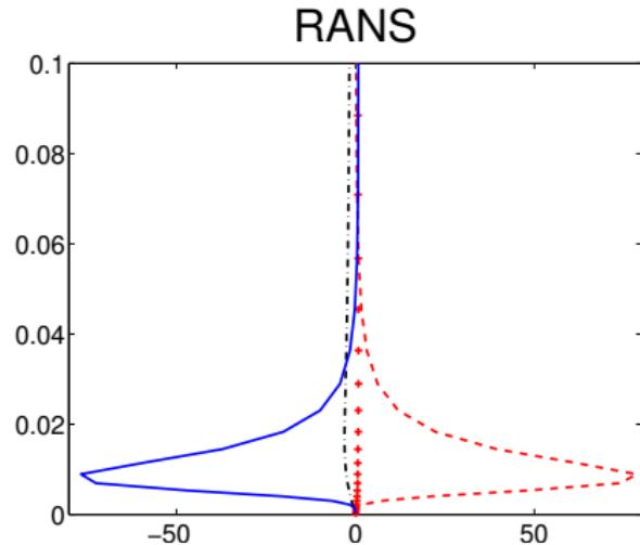
$\text{---: } \frac{\partial}{\partial y} \left( \frac{\nu_t}{\sigma_t} \frac{\partial \langle \bar{t} \rangle}{\partial y} \right); \text{ ---: } \frac{\nu}{\sigma_\ell} \frac{\partial^2 \langle \bar{t} \rangle}{\partial y^2}; \text{ - - -: } -\frac{\partial \langle \bar{u} \rangle \langle \bar{t} \rangle}{\partial x}; \text{ +: } -\frac{\partial \langle \bar{v} \rangle \langle \bar{t} \rangle}{\partial y}; \triangle: \text{---} \frac{\partial \langle v' t' \rangle}{\partial y}.$
