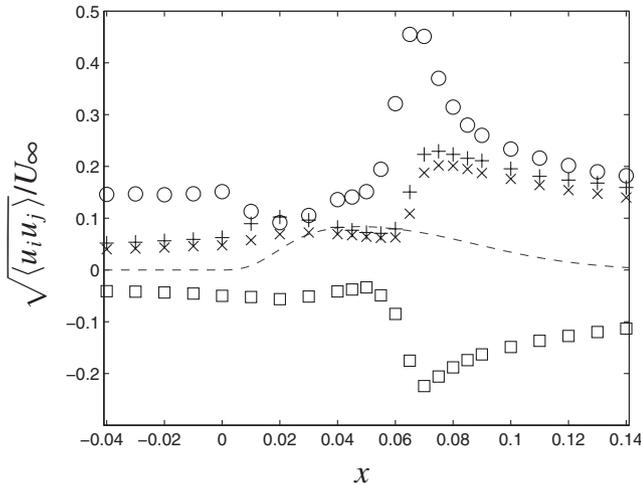
**Fig. 31 Normalized maximum values of the Reynolds stresses:**  $\circ = \sqrt{\langle uu \rangle} / U_\infty$ ;  $\times = \sqrt{\langle vv \rangle} / U_\infty$ ;  $+$   $= \sqrt{\langle ww \rangle} / U_\infty$ ;  $\square = \sqrt{|\langle uv \rangle|} / U_\infty$  (sign restored). The dashed line is the wall profile.
