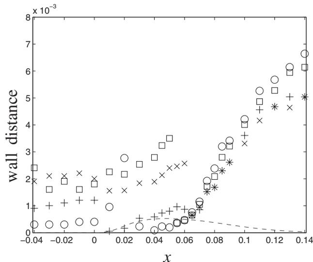
**Fig. 32 Distance from the wall for the maxima of the Reynolds stresses.**  $\circ = \sqrt{\langle uu \rangle} / U_\infty$ ;  $\times = \sqrt{\langle vv \rangle} / U_\infty$ ;  $+$   $= \sqrt{\langle ww \rangle} / U_\infty$ ;  $\square = \sqrt{|\langle uv \rangle|} / U_\infty$ . The dashed line is the wall profile.
