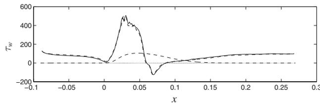
Fig. 10 Wall shear stress: grid 1 (solid line); grid 2 (dashed line).
