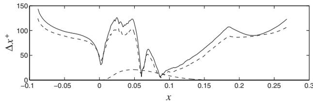
Fig. 11 Streamwise resolutions: grid 1 (solid line); grid 2 (dashed line).
