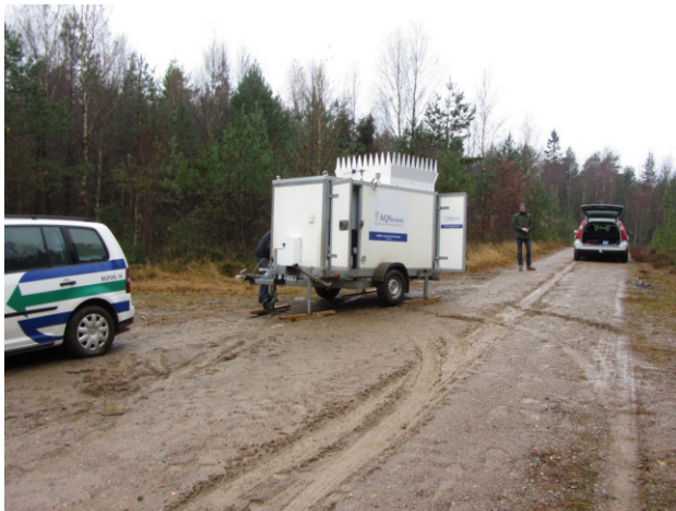
Figure 6.2: Installation of the BRN SODAR.
