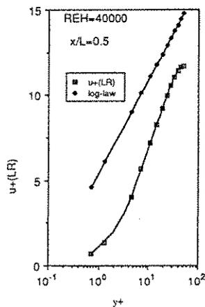
Figure 7. Calculated velocity profile and log-law
