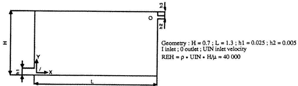
Figure 4. Description of the configuration
