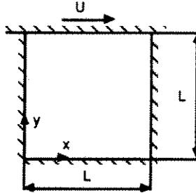
Figure 2. Configuration for the wall-driven square cavity
