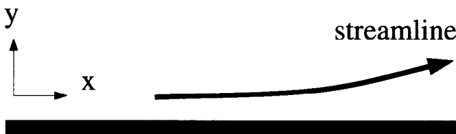
Fig. 2. The streamlines, which in flat-plate boundary layers are along the x -axis, are suddenly deflected upwards (concave curvature) e.g. due to an approaching shock.
