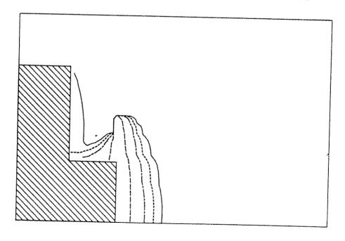
Figure 4. Contours of concentration scaled with mean exit concentration for Case 1,  $< c_{\rm ex,1} >$ . a) Case 1. b) Case 2.
