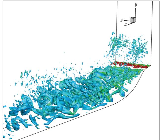
Fig. 18 Hump flow, isosurface of  $Q = -\frac{\partial u_i \partial u_j}{\partial x_i \partial x_j} = 500$  is shown and is colored by vorticity magnitude. Flow from right to left.
