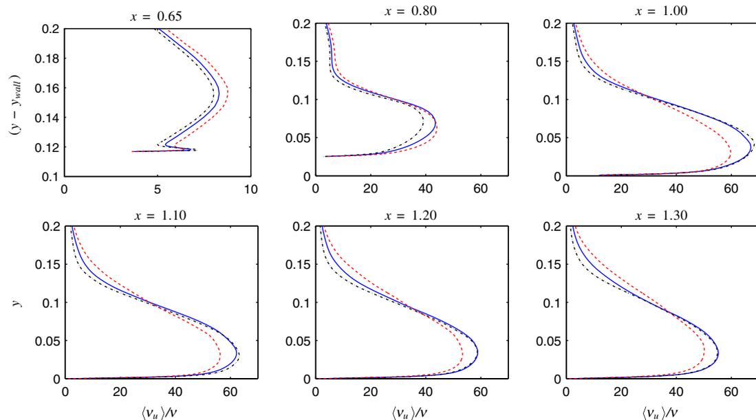
Fig. 17 Hump flow, modeled turbulent eddy viscosity: baseline inlet fluctuations (—; see Fig. 4), 1.5× (baseline inlet fluctuations, ---), 0.5× (baseline inlet fluctuations, · · ·).
