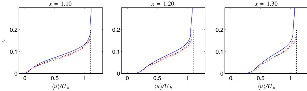
Fig. 15 Hump flow, mean velocity ( $\bar{u}$ ), downstream of reattachment. Vertical dashed thick lines are drawn at  $\langle u \rangle / U_b = 1.10$ : prediction, baseline inlet fluctuations, (—) 2-D PIV experiments (---), and 3-D PIV experiments (· · ·).
