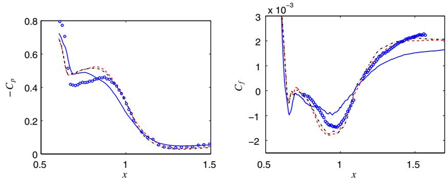
**Fig. 20 Hump flow: a) pressure coefficient, and b) skin friction.** WALE model (—),  $N_k = 128$ ,  $Z_{max} = 0.4$  (---), central differencing scheme (- - -), and experiments (○).
