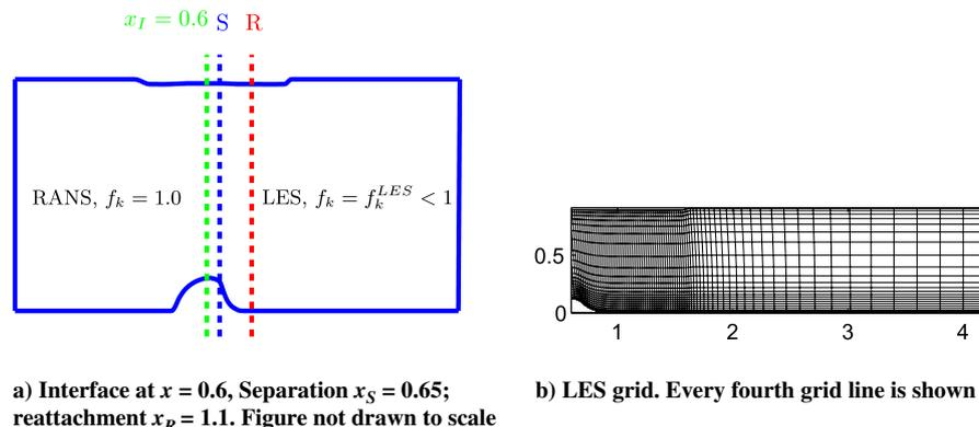
**Fig. 2 Hump flow configuration and grid schematic.**
