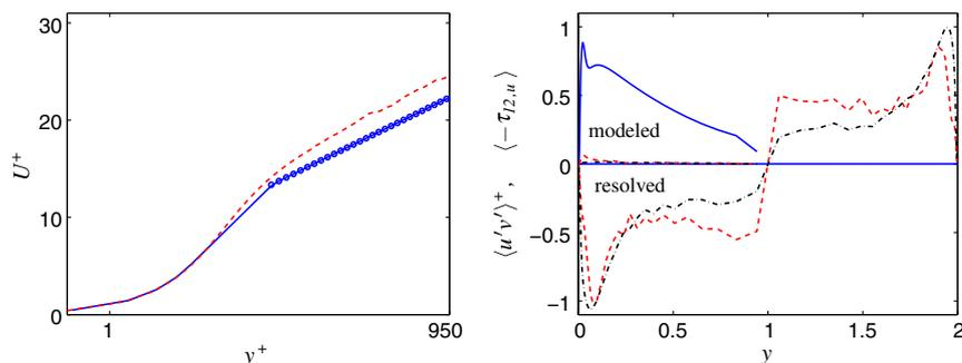
Fig. 5 Channel flow; time-averaged streamwise ( $U$ ) velocity as well as resolved and modeled (opposite sign) shear stresses:  $x = 0.19$  (—),  $x = 1.25$  (— —), and  $x = 3$  (- - -). The log law is plotted in symbols.
