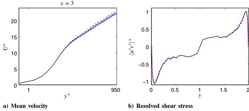
**Fig. 9** Channel flow. Sensitivity to  $f_k$  in the LES region. Mean velocity and resolved shear stresses at  $x = 3$  for  $f_k = 0.4$  (—),  $f_k = 0.2$  (---), and  $f_k = 0.6$  (- - -).
