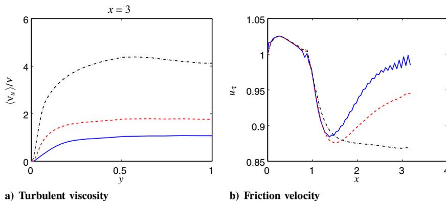
Fig. 8 Channel flow, sensitivity to  $C_S$ , see Eq. (11): a) Turbulent viscosity at  $x = 3$ , and b) friction velocity for  $C_S = 0.07$  (—),  $C_S = 0.1$  (— —), and  $C_S = 0.2$  (---).
