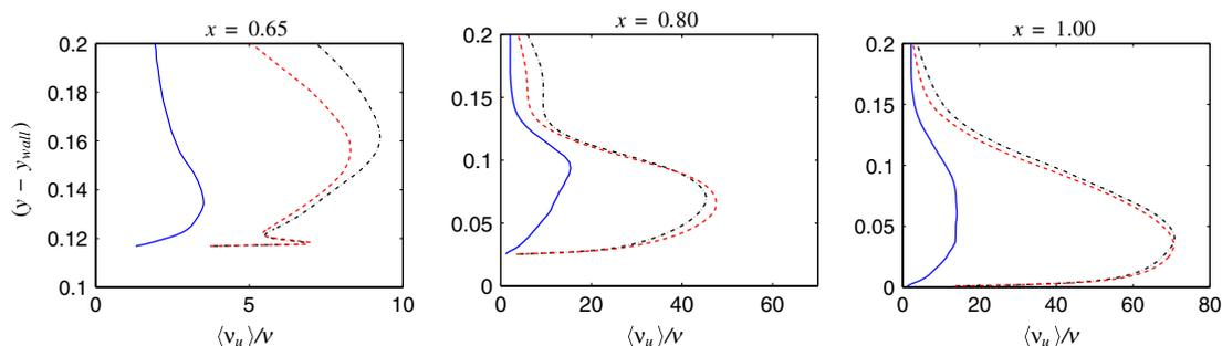
**Fig. 23 Hump flow, turbulent viscosity: WALE model (—),  $N_k = 128, Z_{\max} = 0.4$  (---), and central differencing scheme (· · ·).**
