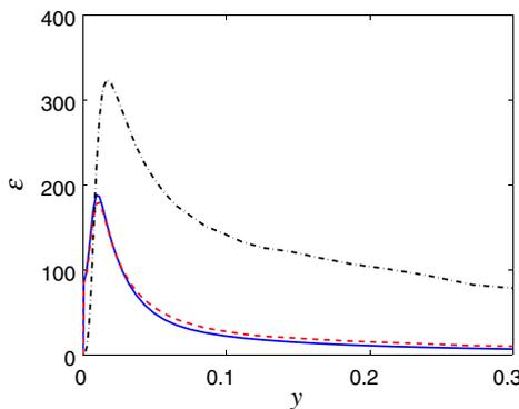
**Fig. 11** Channel flow; dissipation  $\epsilon$  at  $x = 0.5$  (—);  $\epsilon$  immediately upstream the interface at  $x = 0.9$  (---); and  $\epsilon_{inter}$  (— · —); see Eq. (12) with  $C_s = 0.07$ .
