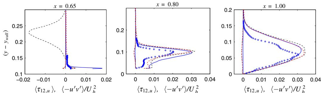
**Fig. 22 Hump flow, resolved and modeled shear stresses: WALE model (—),  $N_k = 128, Z_{\max} = 0.4$  (---), central differencing scheme (· · ·), and 2-D PIV experiments (○).**
