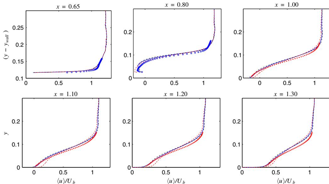
Fig. 14 Velocity ( $\bar{u}$ ): baseline inlet fluctuations (—) (see Fig. 4), 1.5× (baseline inlet fluctuations) (---), 0.5× (baseline inlet fluctuations) (---), 2-D PIV experiments (○), and 3-D PIV experiments (+).
