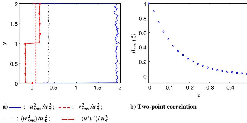
Fig. 3 Channel flow, prescribed synthetic Reynolds stresses at the RANS-LES interface.
