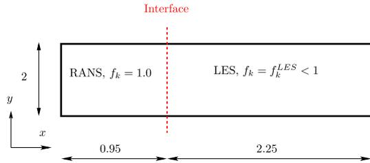
**Fig. 1 Channel flow configuration. The interface separates the RANS and the LES regions.**
