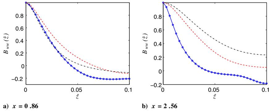
**Fig. 19 Hump flow, two-point correlations:**  $y - y_{wall} = 0.00085$  (—),  $y - y_{wall} = 0.014$  (---), and  $y - y_{wall} = 0.10$  (- - -). Markers indicate the grid spanwise resolution.
