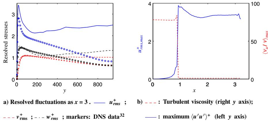
Fig. 6 Channel flow: a) resolved normal resolved RMS fluctuations at  $x = 3$ , and b) maximum  $u_{rms}^+$  and  $\langle \nu_u / \nu \rangle$  versus  $x$ .
