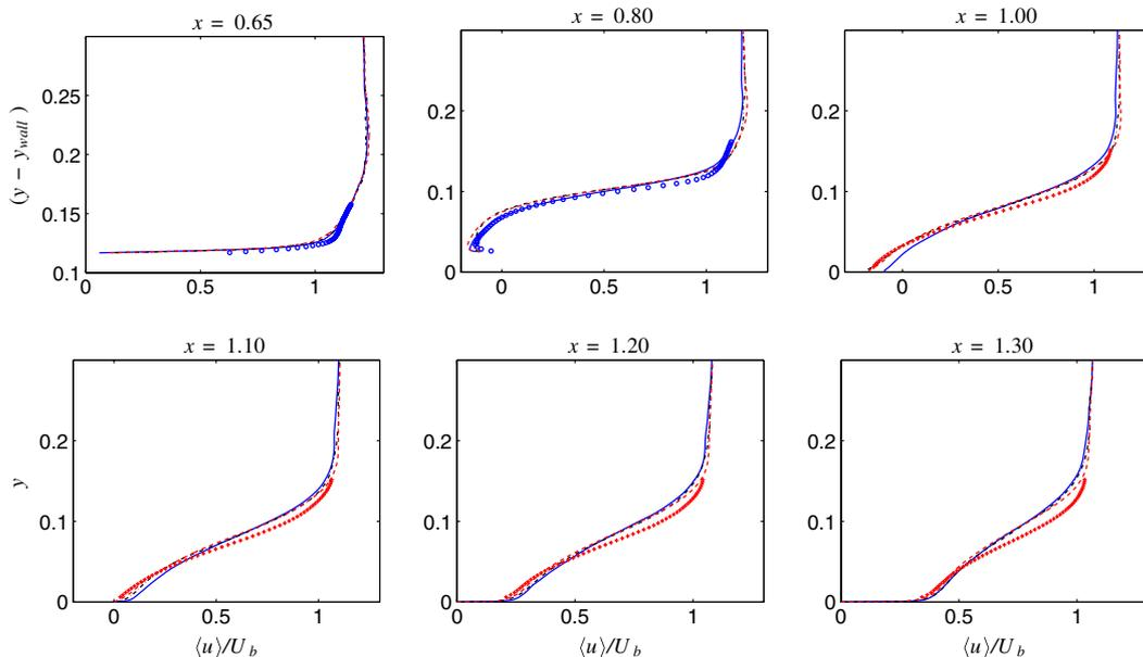
**Fig. 21 Hump flow, mean velocity  $\langle \bar{u} \rangle$ :** WALE model (—),  $N_k = 128$ ,  $Z_{max} = 0.4$  (---), central differencing scheme (- - -), 2-D PIV experiments (○), and 3-D PIV experiments (+).
