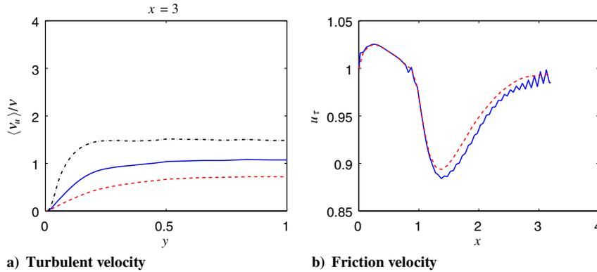
**Fig. 10** Channel flow; sensitivity to  $f_k$ : a) turbulent viscosity at  $x = 3$ , and b) friction velocity for  $f_k = 0.4$  (—),  $f_k = 0.2$  (---), and  $f_k = 0.6$  (- - -).
