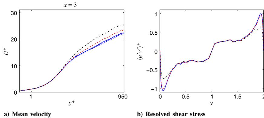
Fig. 7 Channel flow, sensitivity to  $C_S$ , see Eq. (11),  $x = 3$ : a) mean velocity, and b) resolved shear stresses for  $C_S = 0.07$  (—),  $C_S = 0.1$  (— —), and  $C_S = 0.2$  (---).
