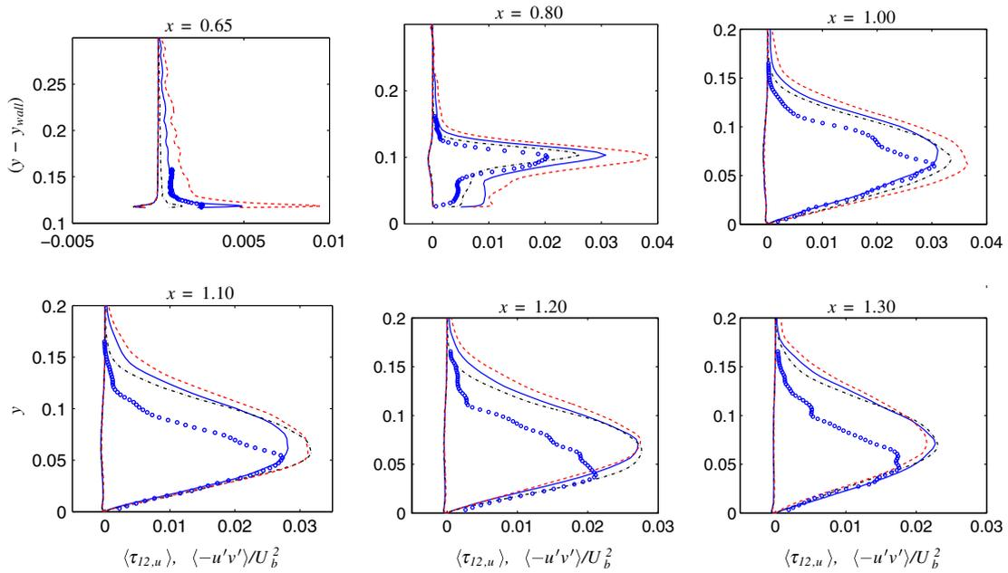
Fig. 16 Hump flow, resolved and modeled turbulent shear stresses: baseline inlet fluctuations (—, see Fig. 4), 1.5× (baseline inlet fluctuations, ---); 0.5× (baseline inlet fluctuations, · · ·); 2-D PIV experiments (○).
