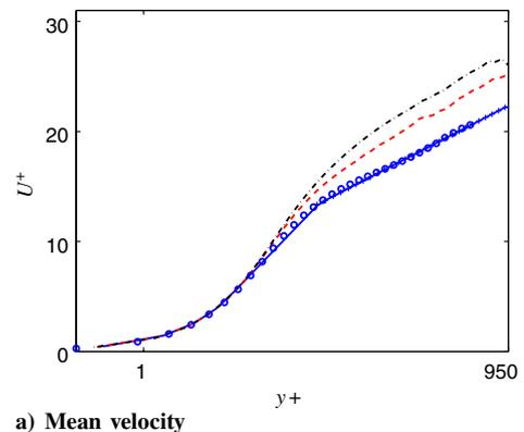
**Fig. 12** Channel flow. Coarse grid resolution in spanwise direction,  $N_k = 32$ ,  $f_k = 0.4$ ,  $C_s = 0.07$ . (—)  $x = 0.19$ ; (---)  $x = 1.25$ ; (- - -)  $x = 3$ ; DNS data (○) [33]; and fully developed channel flow (+).
