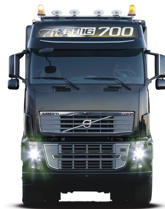
Figure 1.0.1: Roof bow carrying lights on top of a truck. Picture from AB Volvo Groups official gallery, with permission.
