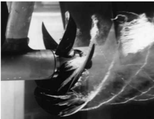
Cavitation downstream of a propeller [ref]
