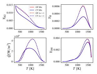
Comparison of Cantera and OpenFOAM solutions for 1D freely propagating flame using unity-Lewis and mixture-averaged transport.
