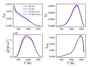
Comparison of Cantera and OpenFOAM solutions for 1D freely propagating flame with Soret effect.
