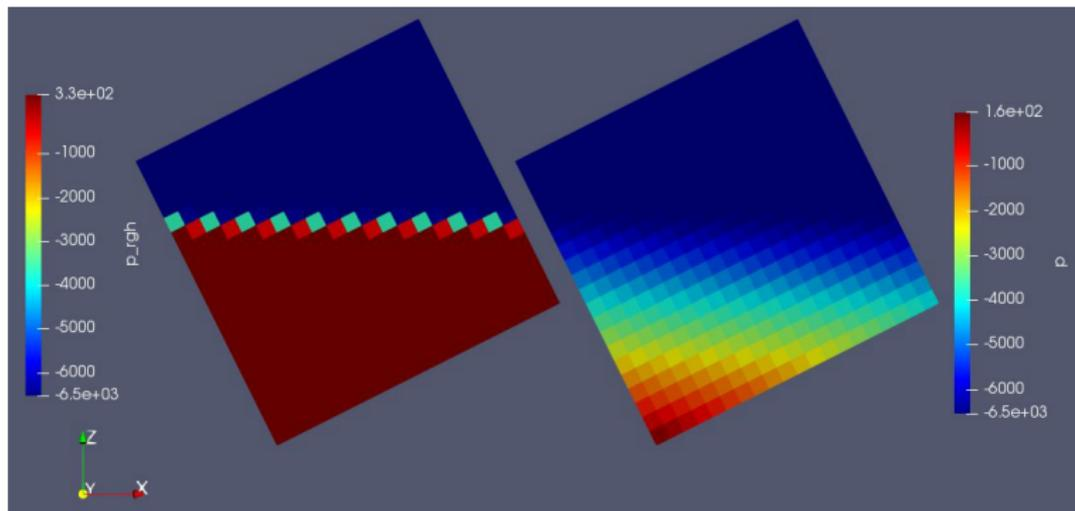
Dynamic ( $p\_rgh$ ) and total pressure ( $p$ ) fields for a static free surface discretised with standard Gauss Laplacian scheme in InterIsoFoam.
