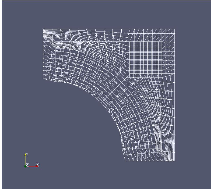
The small arc has a radius of 0.5m, the bigger one 0.75m, the complete height and length are 0.8m and the width is 0.5; it is a scale 1:10.
