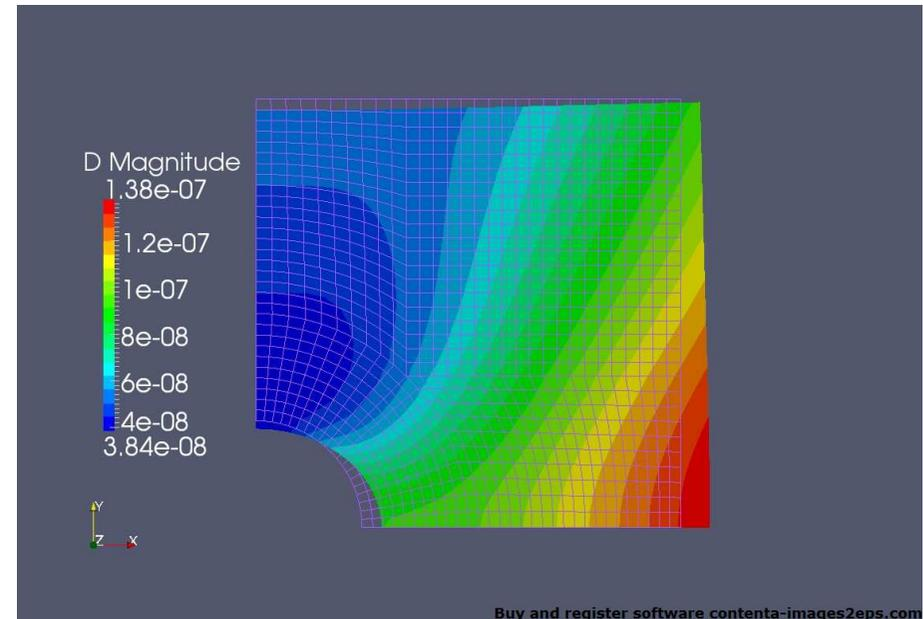
Loaded plate with a hole. Equivalent stresses shown and displacement with a scale factor of  $1e6$  (WarpByVector filter used).
