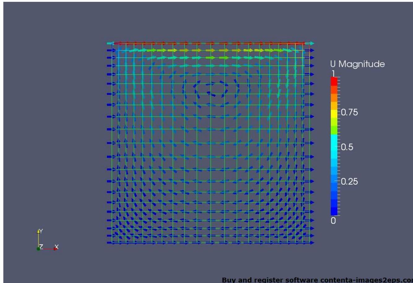
CavityGrade case meshing and solution with Glyph filter showing velocity vectors and magnitude.
