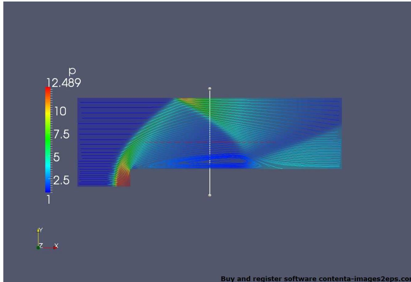
Streamlines and pressure waves for the forwardStep case.
