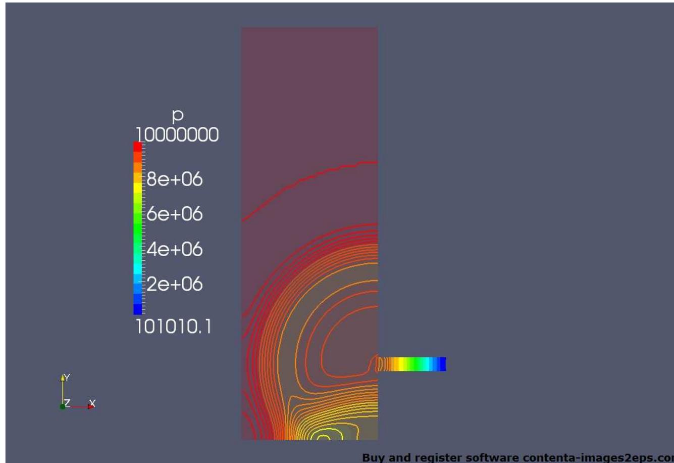
Contour lines for pressure waves shown for decompression tank case.
