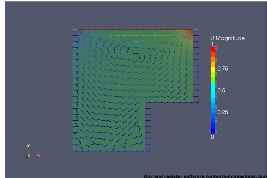
Cavity case with extracted block. Cavity solution velocity field mapped onto cavityClipped case and final solution for the case.(Glyph filter used)
