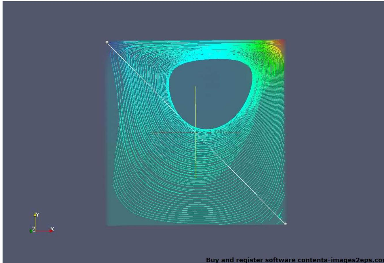
Cavity case with High Reynolds number flow. StreamTracer filter used to visualise the results.
