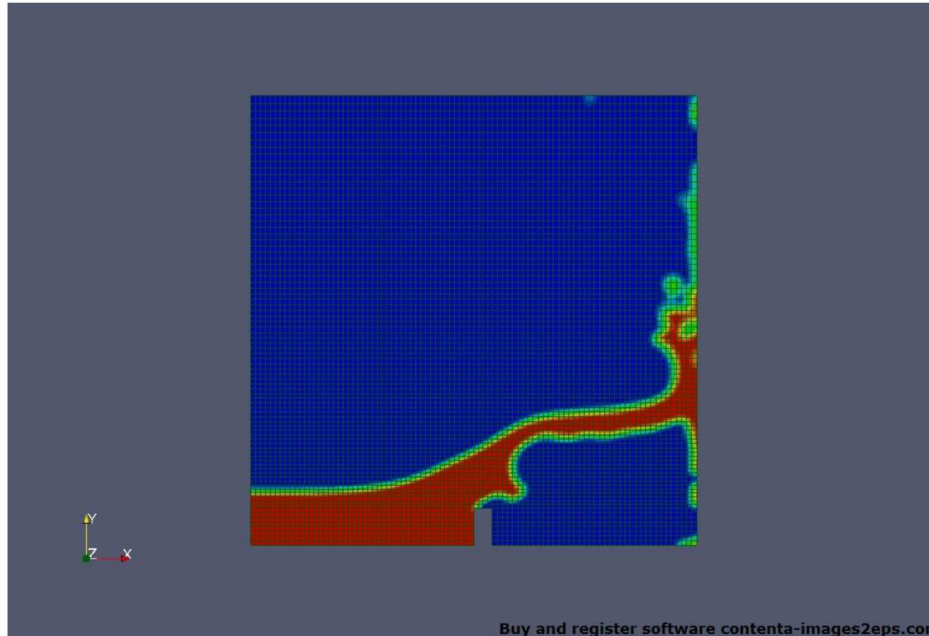
DamBreak with fine mesh. Alpha1 fraction distribution shown at the last step calculated.
