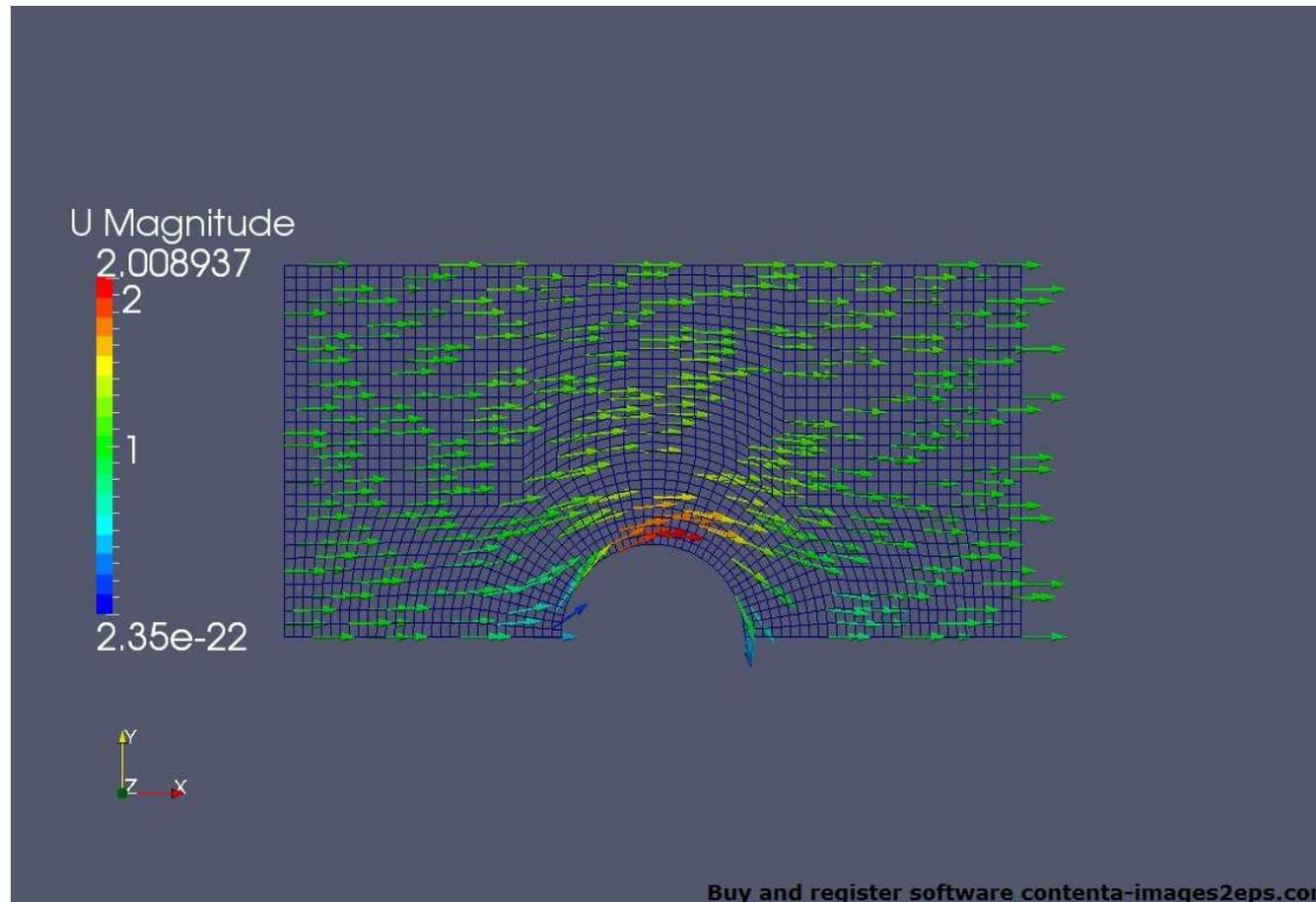
Glyph filter used to show the flow around the cylinder. Vectors are colored with velocity magnitude.
