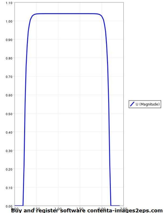
Magnetohydrodynamic flow of a liquid, velocity distribution over the line for  $B=20T$  is shown.
