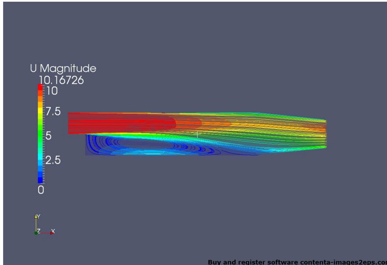
Streamlines in a steady turbulent flow over a backward-facing step.
