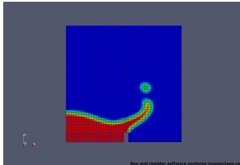
DamBreak case with alpha1 fraction distribution shown in different time steps.
