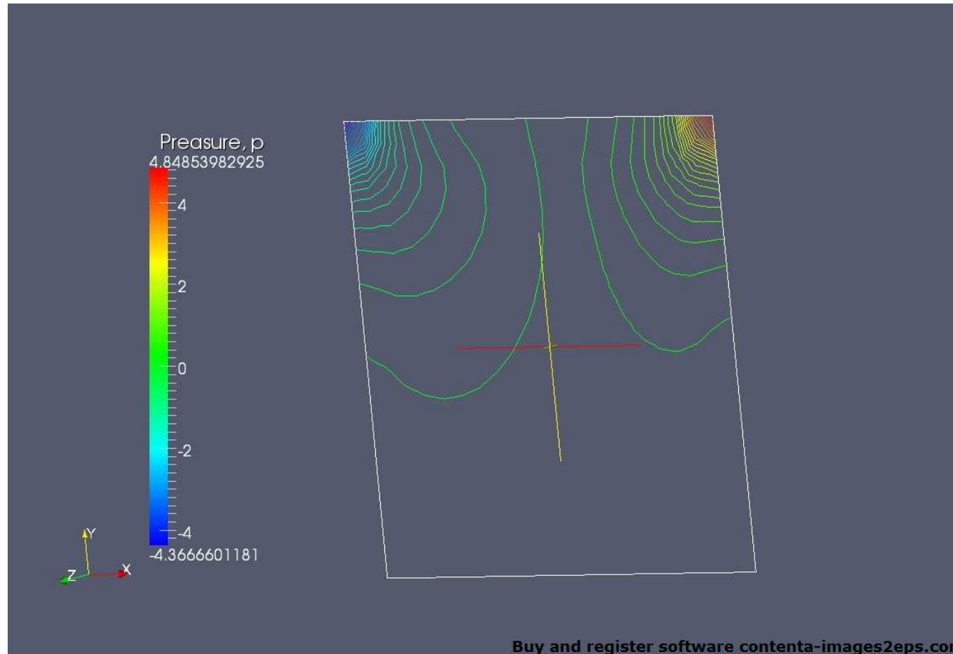
Cavity case solution with Slice filter and contour lines for pressure distribution.
