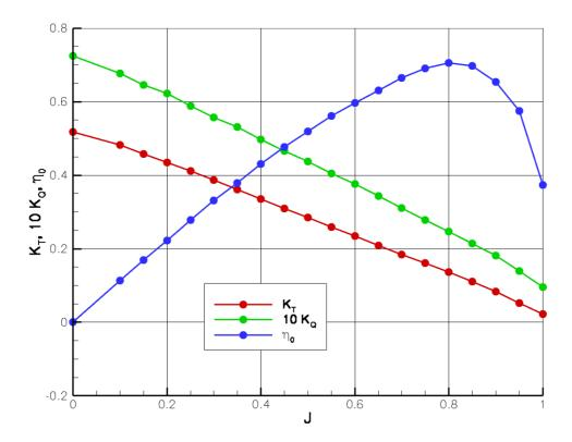
For a prescribed thrust and/or an advance ratio parameter knowing the advance speed U and ratio J from the propeller rotation speed (n or  $\Omega$ ),  $K_Q$  is obtained form the performance curve and the propeller torque  $\mathbf{Q}$  can be deduced from the propeller thrust  $\mathbf{T}$  as:
