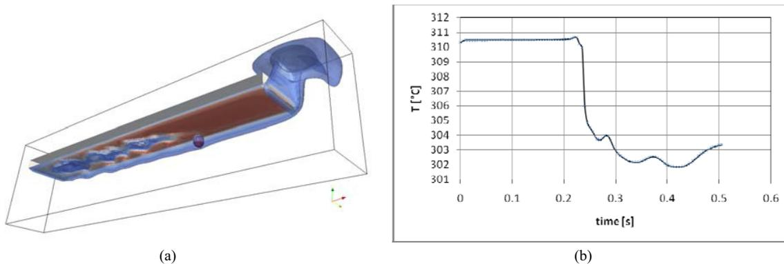
Effect of sliding bubble on thermal boundary layer due to free convection from a inclined and immersed flat plat as predicted by OpenFOAM. (a) Contour plot of thermal boundary layer. (b) history plot of wall temperature at a point along the plate centreline.
