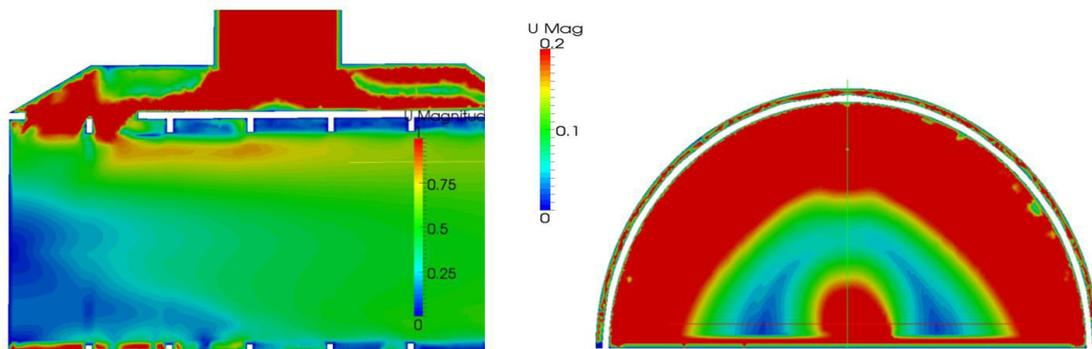
Figure 1: Velocity contours near in the Heat Exchanger. The tubesheet is modelled by a porous medium.
