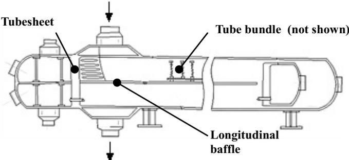
Figure 2: Configuration of the Heat Exchanger.
