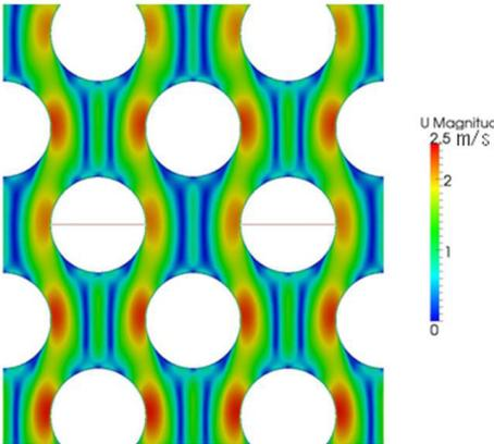
Figure 3: Cross sectional velocity field of the salt flow in the tubesheet.
