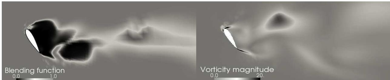
Figure: Evolution of vorticity magnitude and blending function for hybrid scheme shortly after initialization with results obtained by unsteady RANS
