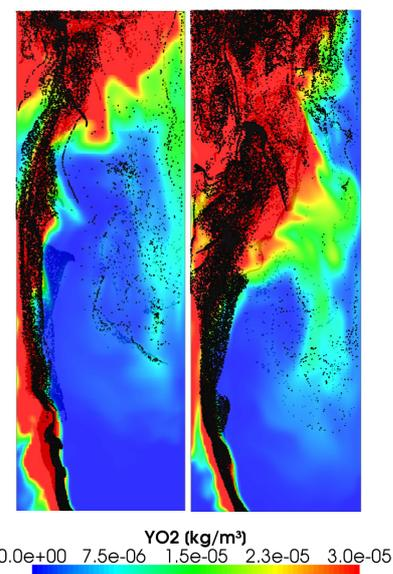
**Fig. 1:** Oxygen distribution in a gassed bioreactor [2].
