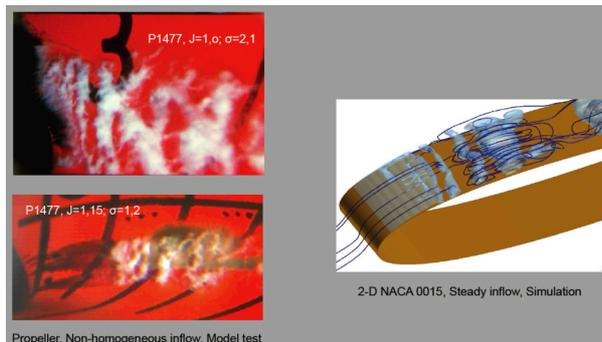
**Figure 1.** Vortex group cavitation downstream a mainly glassy sheet on a propeller during model testing and simulated by Large Eddy Simulation, LES, at a 2D foil with some streamlines indicated.
