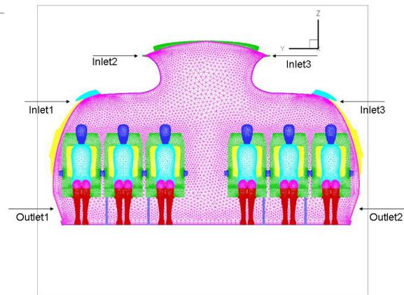
Fig 1.: Volume Mesh of a segment of an A-320 cabin model
