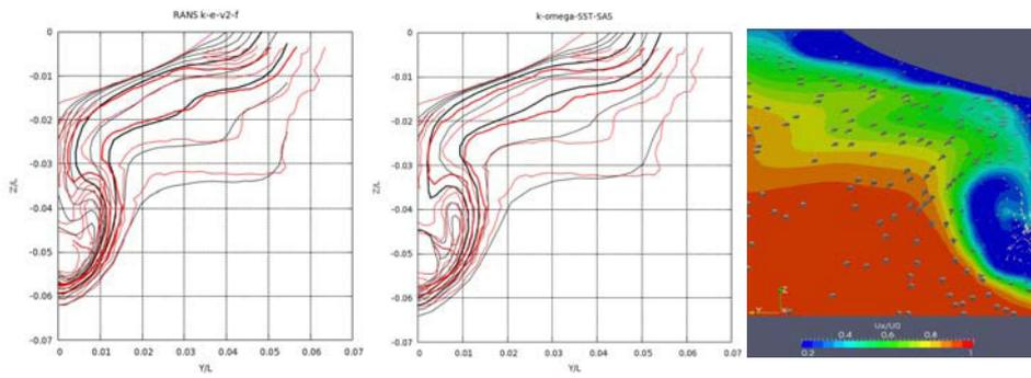
Fig.1 Wake field in the propeller disk. Red curves- KRISO measurements, black- OpenFoam simulations, colour picture- instantaneous field obtained by the hybrid method.
