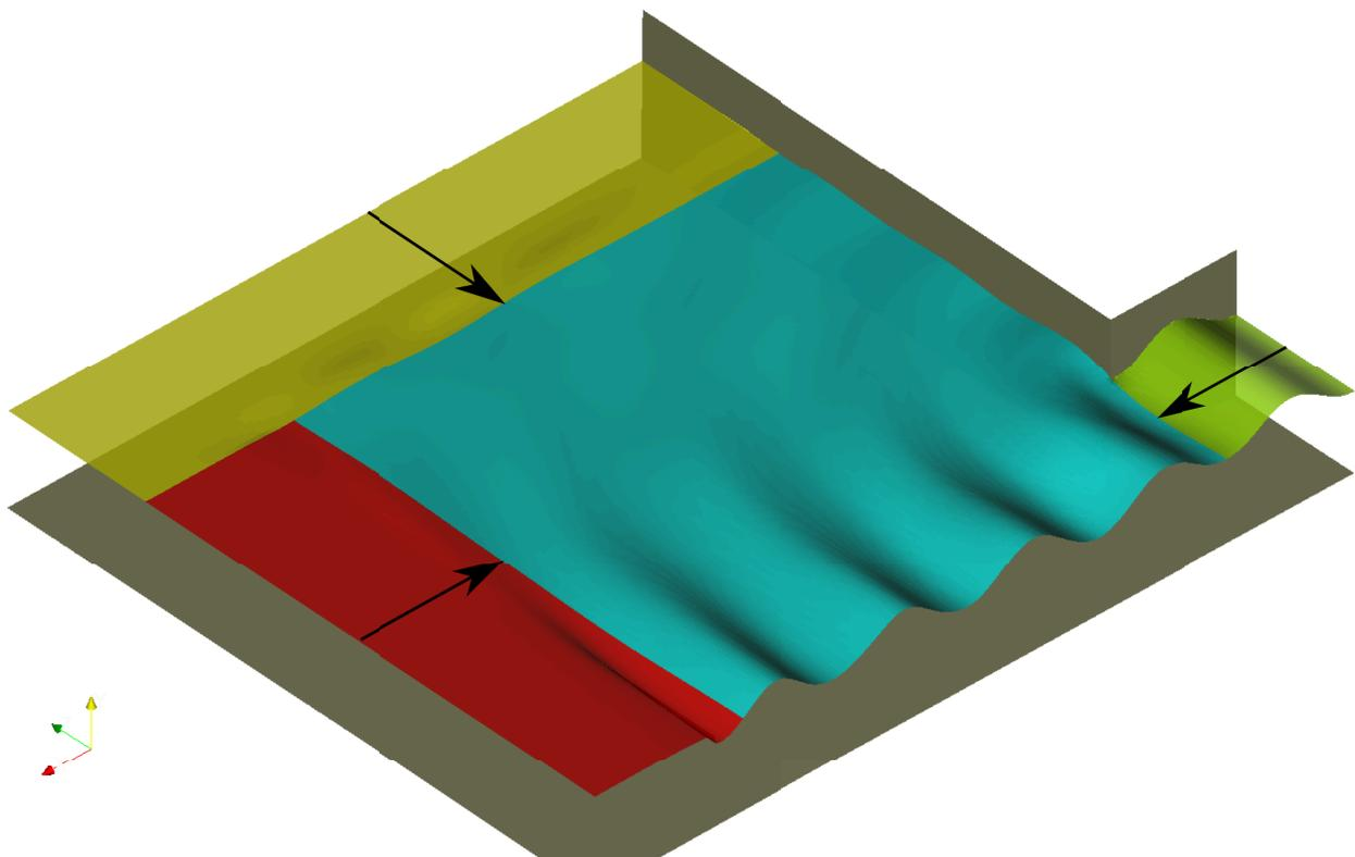
Figure 1: Diffraction of surface water waves through a breakwater gap. The three relaxation zones are the green, yellow and red areas respectively. Arrows indicate the direction of zero relaxation.
