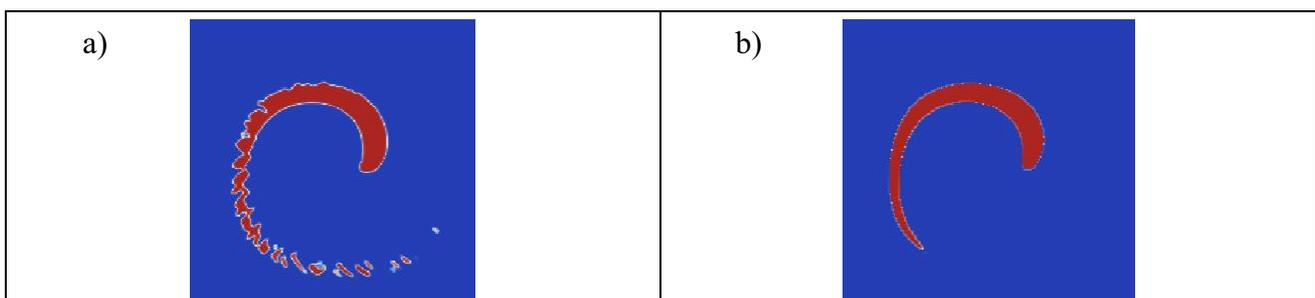
Figure 1: Performance of interFoam (a) and interCLSVOFFoam (b) on the circle in a vortex testcase
