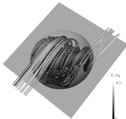
Vortex structures obtained from LES velocity field
