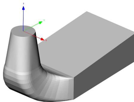
Figure 1.: elbow draft tube
