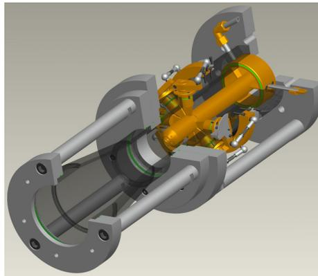
Figure 1: Swirl generator with conical diffuser
