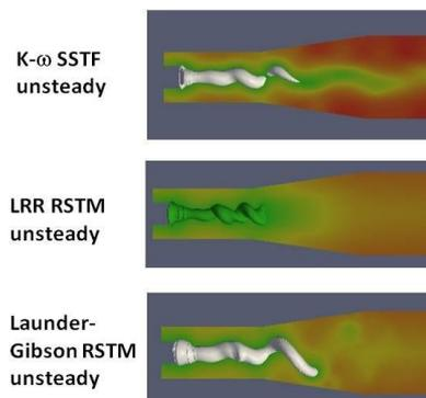
Figure 2: Simulation of vortex rope – applied are different turbulence models
