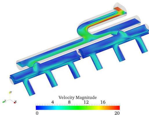
Figure 1: Flow field in the header configuration.
