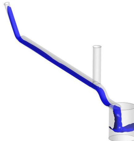
Figure 2: Volume fraction of the liquid mixture in the finger pipe.
