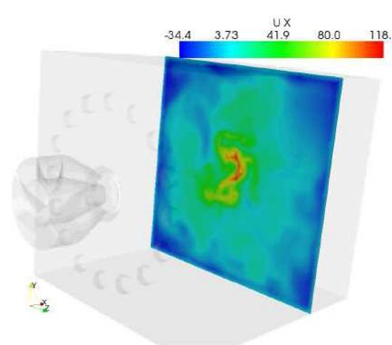
Figure 2: LES snapshot of the streamwise velocity field [m/s] in a swirling jet. The swirler geometry is represented in light grey.
