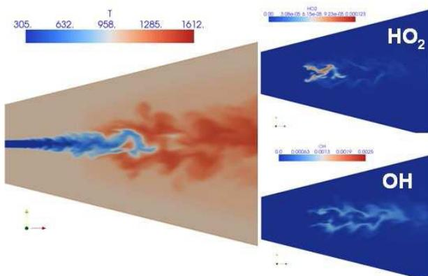
Figure 1: LES of auto-ignition of a high speed hydrogen jet discharging in hot oxidant using detailed chemistry.
