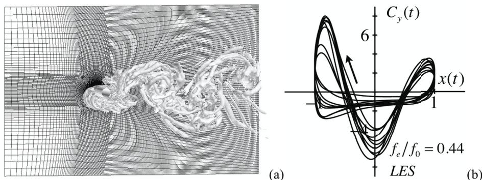
Figure 1. In (a) a perspective view of the flow field around an oscillating cylinder with dimensionless excitation frequency  $f_e/f_0=1.00$  in term of iso-surfaces of the second invariant of the velocity gradient. In (b) the Lissajous curve of the lift force coefficient,  $C_y(t)$ , versus the displacement of the cylinder,  $x(t)$ , is displayed.
