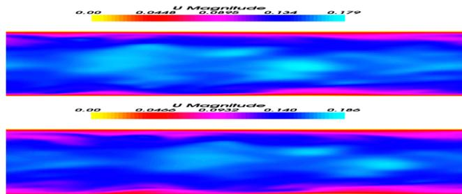
Fig.3 Qualitative effect of air particles in near wall region (up: w/o particle effects, Down: with particle effects)
