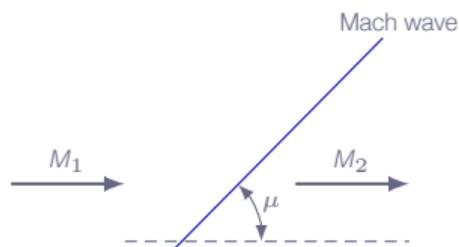
No substantial changes of flow properties over a single Mach wave
