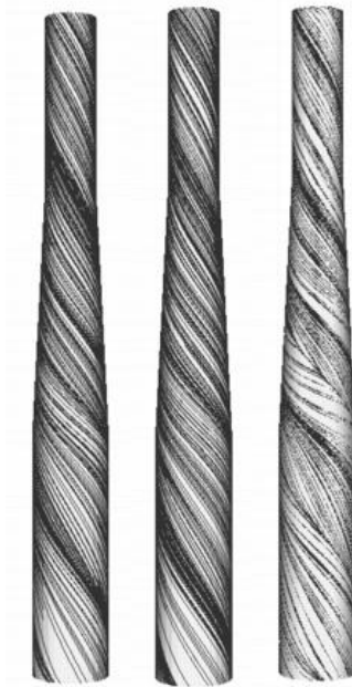
Figure 5 Smearlines for cases 1, 2 and 3 respectively. The use of wall functions and a coarser mesh in case 1 and 2 makes the irregular structures less evident.
