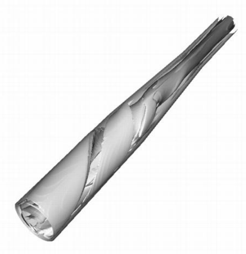
Figure 2 Iso-surface of normalised helicity at a level of -0.8.
