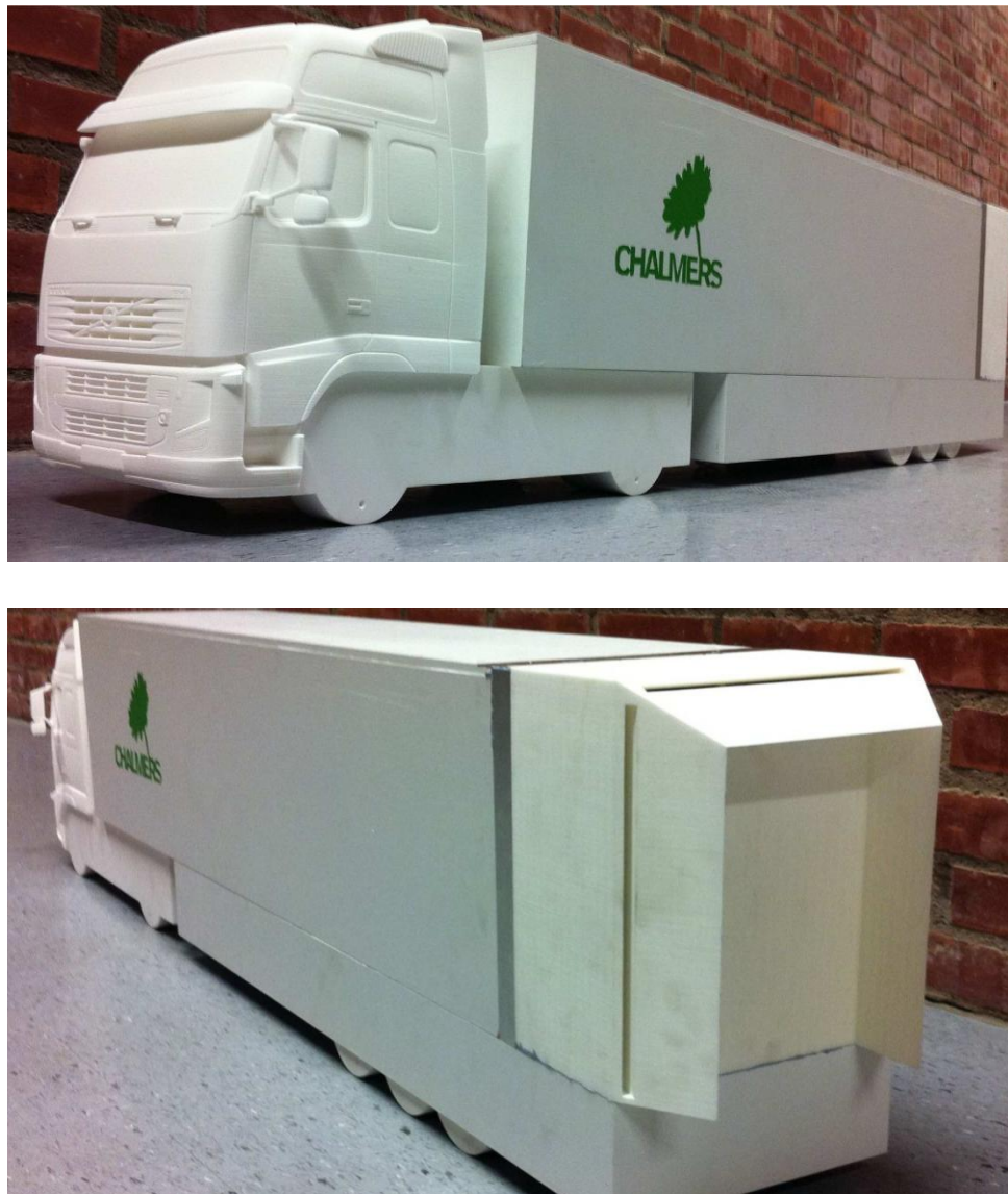
Figure 1: A front and rear view of a 1:10 experimental scale model of a VOLVO FH16 with flaps. The slots are also shown in the rear view.
