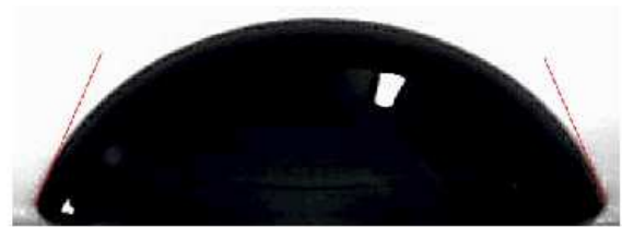
Figure 4: Measurement of the static contact angle.
