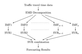
Fig. 7. Process schema of EMD-SVR method.
