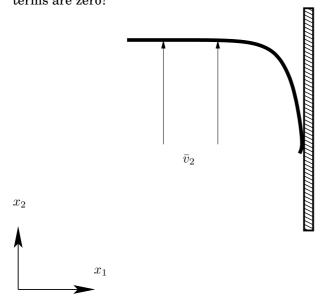
T3. a) Consider natural convection in the figure below. The convective velocity field is negligible. Is the stratification stable or unstable? Show that the Reynolds stress model faithfully can model the stratification.
