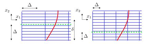
Grid (in blue) and a velocity profile (in red). RANS-LES interface is shown by the dashed-green line.
