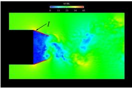
In the figure above the rear part of a simplified truck is shown. Flaps have been added (marked in red) and at the beginning of the flaps, the pulsating jets (marked with an I) are located. The figure shows the instantaneous velocity field (green: high velocity; blue: low velocity).
