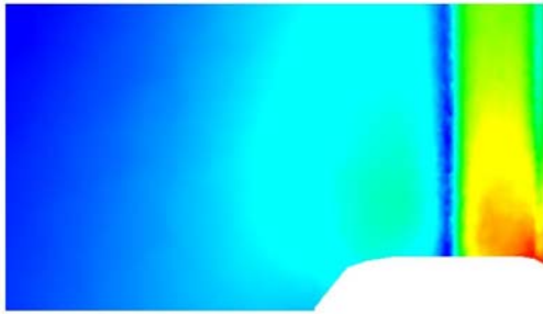
Figure 6. a- Mean tangential velocity – k-\epsilon (m/s)
