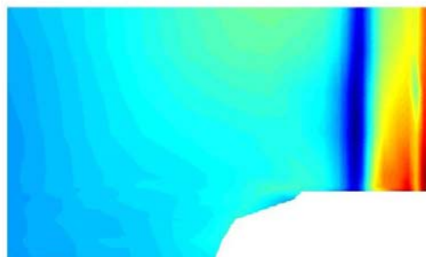
Figure 9. a- Mean tangential velocity – experimental (m/s)
