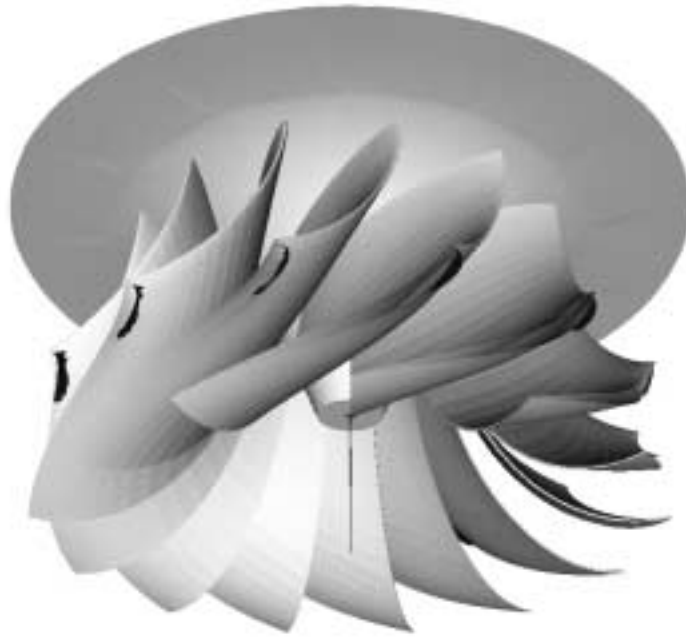
(a) Pressure coefficient iso-surface, C_p = -0.25 (colored dark), operating point 1.
