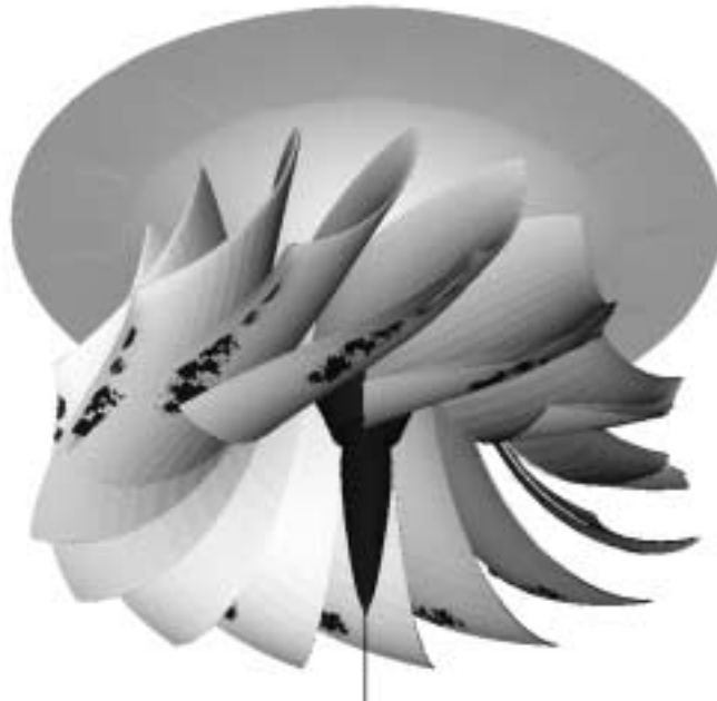
(b) Pressure coefficient iso-surface, C_p = -0.3 (colored dark), operating point 2.
