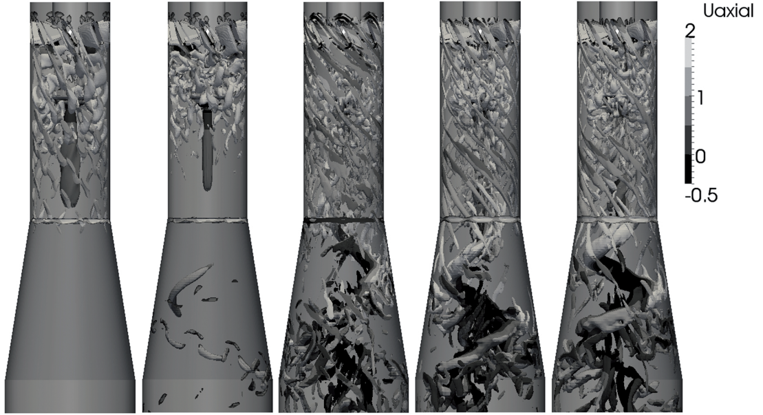
Figure 3.3.6: Isosurface of the second invariant of the velocity gradient tensor (colored by axial velocity in [\frac{m}{s}] ). The axial velocity is positive in flow direction, i.e. from top to bottom. From left to right: k-\epsilon , k-\omega SST, k-\omega SST SAS, Spalart-Allmaras DDES and Spalart-Allmaras IDDES.
