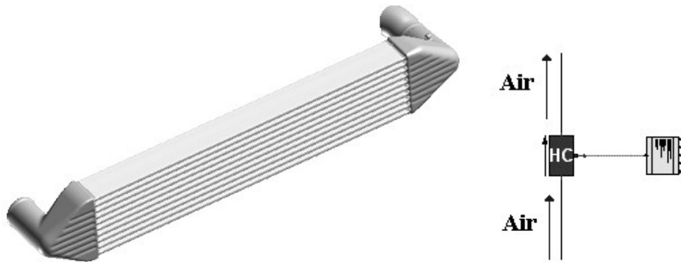
Figure 6.9 Charge Air Cooler, represented in CAD and Flowmaster respectively
