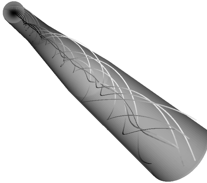
FIGURE 4.0.1: Streamlines and inlet pressure distribution where dark color represents low pressure. Particles are released along a radial line at a fixed tangential position at the inlet and are traced along the steady flow.
