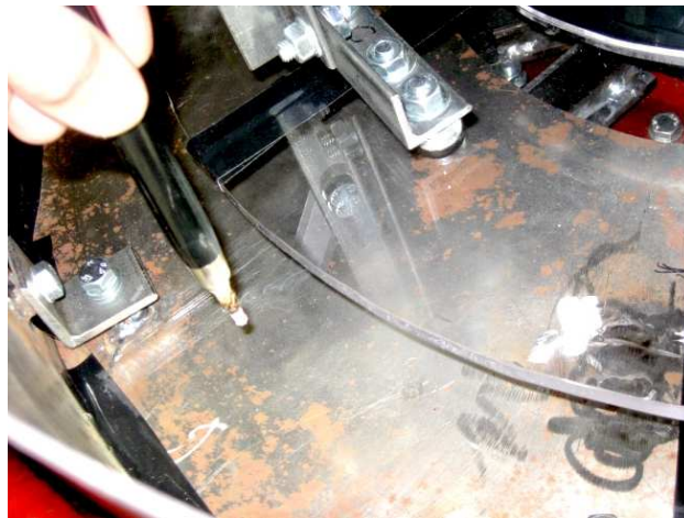
Figure 2.2: Smoke pen at the inlet of the generator
