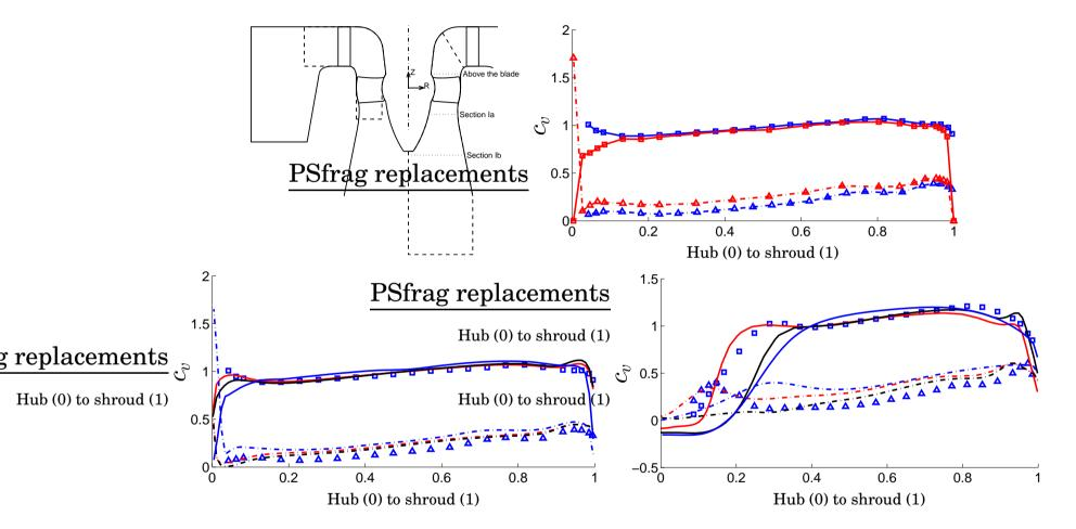
Squares: measured axial velocity. Triangles: measured tangential velocity. In (a) the colors correspond to two different measurements. In (b) and (c): Blue curve: quasi-steady draft tube, Black curve: runner without hub clearance, Red curve: runner with hub clearance.
