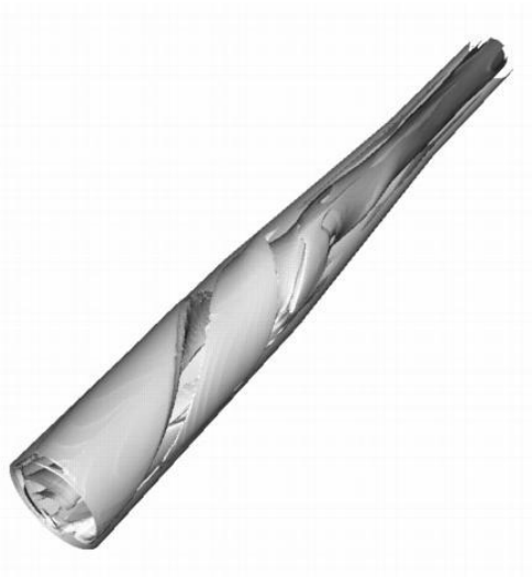
Figure 2 Iso-surface of normalised helicity at a level of -0.8.
