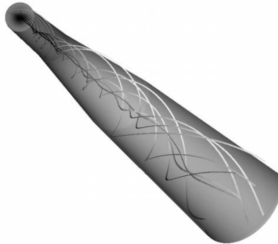
Figure 1 Streamlines and inlet pressure distribution where the dark colour represents low pressure. Particles are released along a radial line at a fixed tangential position at the inlet and are traced along the steady flow.
