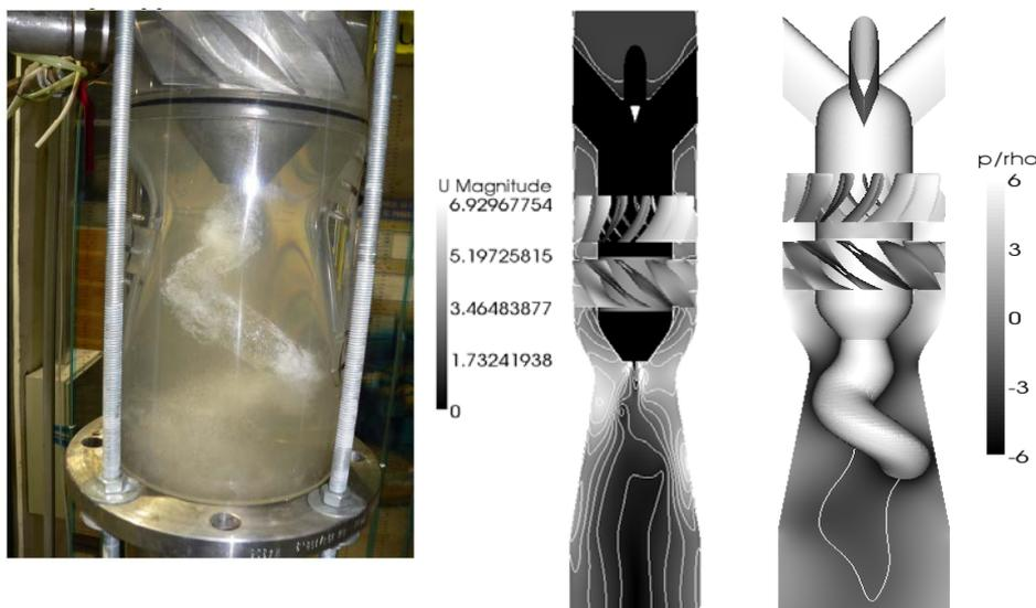
**Fig. 9:** The precessing vortex rope visualized in the experimental test section (left), and snap-shots of the velocity (centre) and pressure field (right) predicted by the numerical simulations in OpenFOAM. For the pressure snap-shot, the iso-surface visualizes a surface of constant pressure, while the iso-line shows where the axial velocity is zero.
