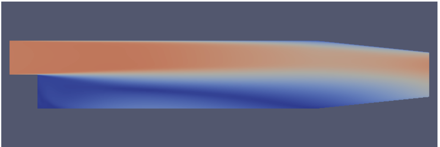
Velocity at final time step with kOmegaSST (using the same solver and case):
